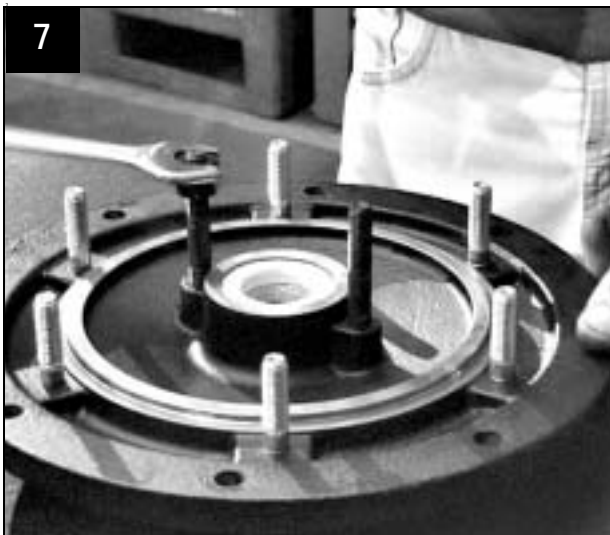
7 Fit studs in cover for pump housing
