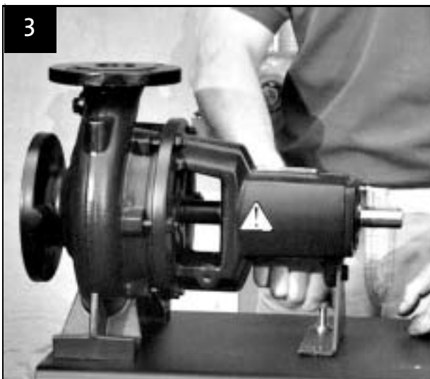
Fasten pump including support with screws
