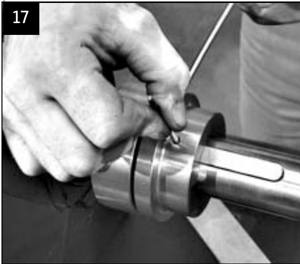
Tighten screw in coupling half
