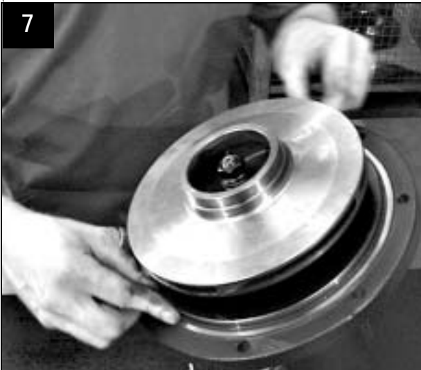
Fit O-ring on cover for pump housing
