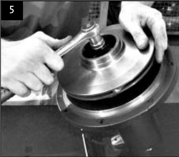
Tighten impeller nut
