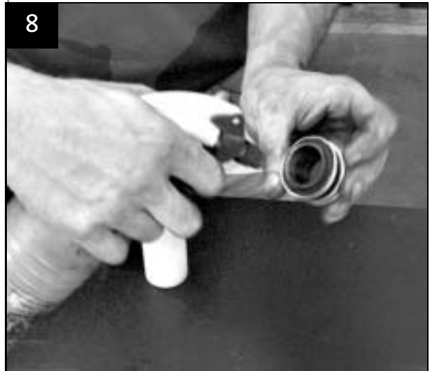
Lubricate rotating part of shaft seal with soapy water
