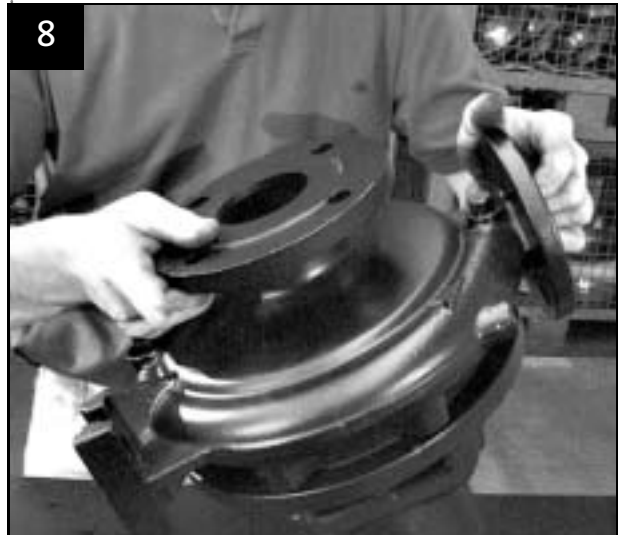
Mount pump housing on cover for pump housing
