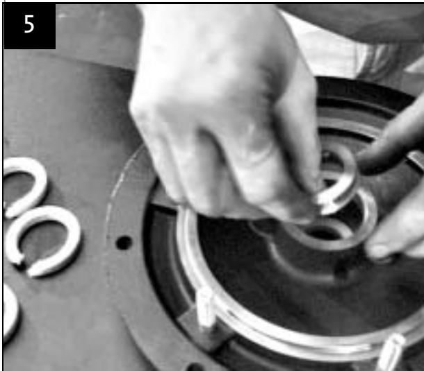
5 Fit lantern ring in cover for pump housing
