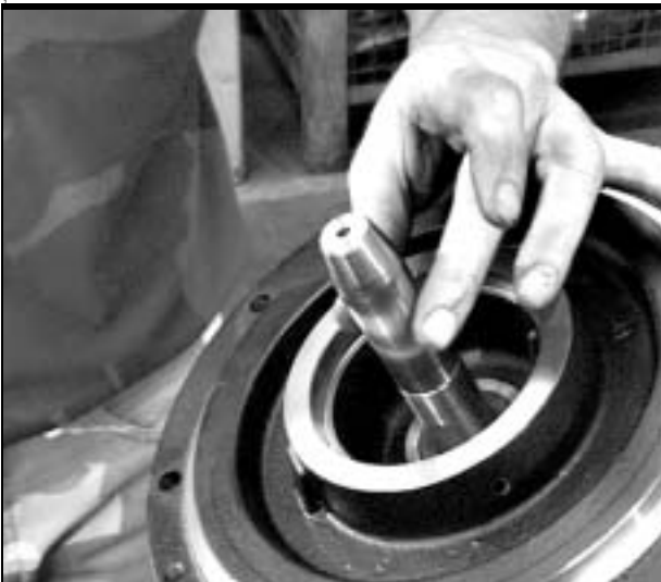
Fit protecting sleeve on shaft
