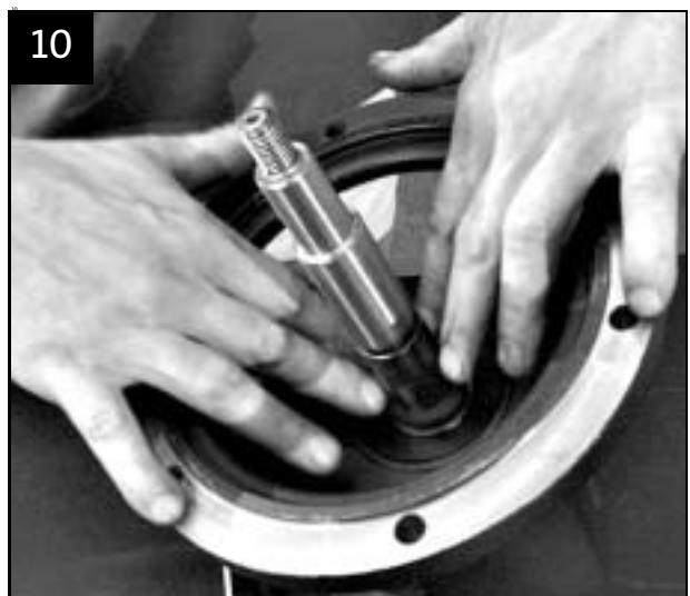
Lubricate second thrower with soapy water and fit it on shaft
