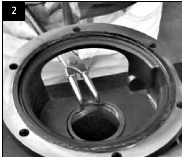
Fit circlip in bearing housing
