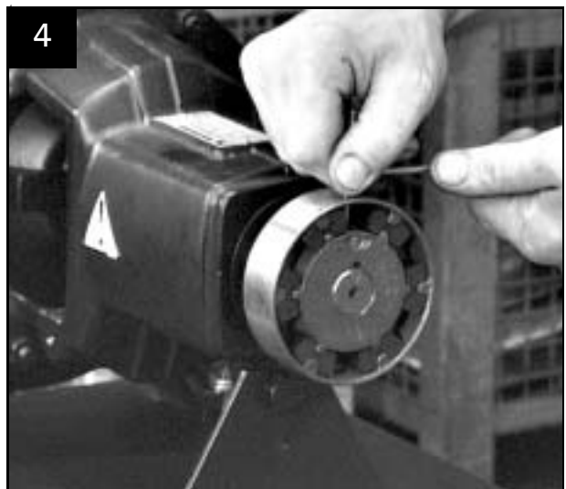
Fit complete coupling half on pump shaft
