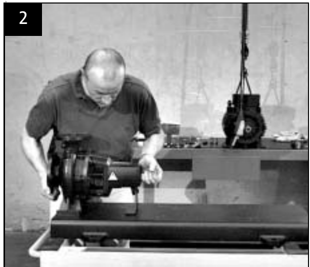
Place pump on base plate
