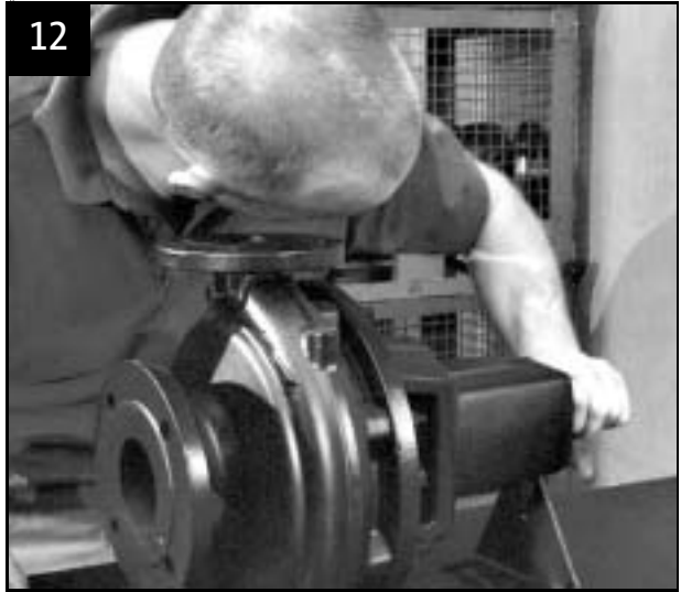
Check free rotation of impeller
