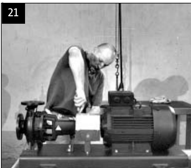
Tighten screws in coupling guard
