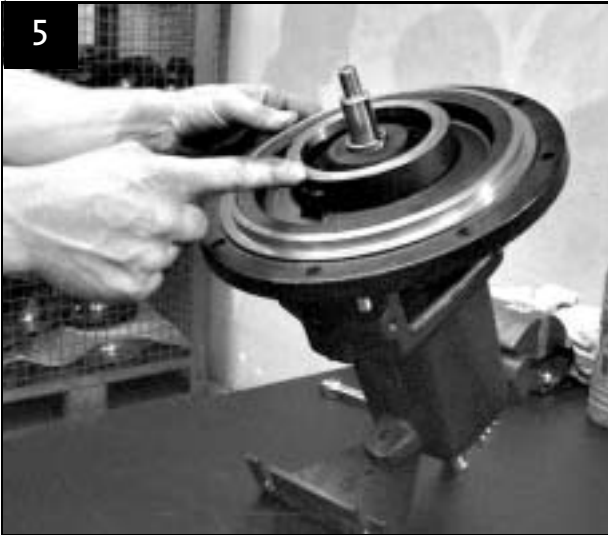
Keep drain hole for shaft seal downwards
