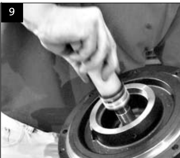
Press shaft seal into bottom position
