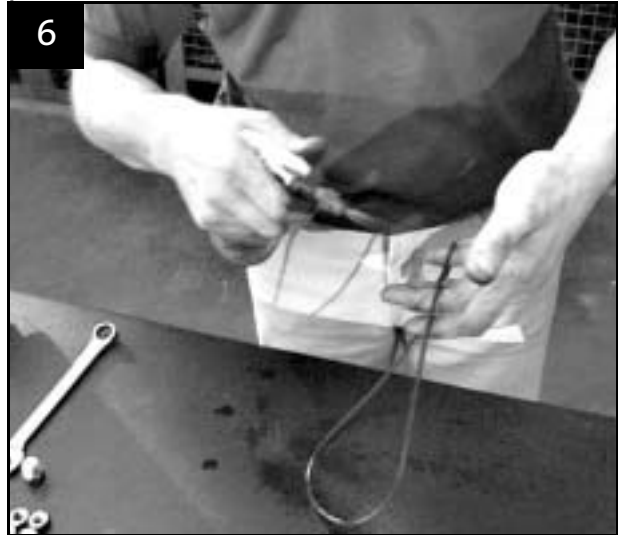
Lubricate O-ring for pump housing and cover for pump housing with soapy water
