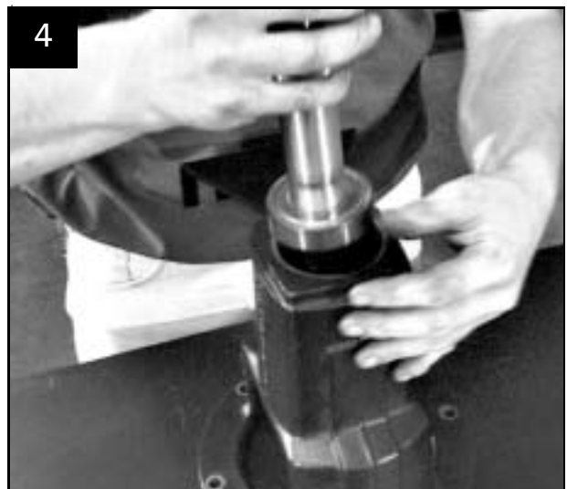
Fit shaft with bearings into bearing housing
