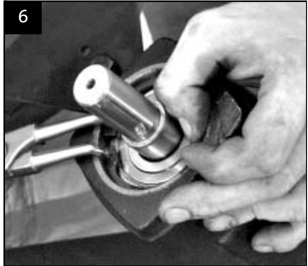
Fit second circlip
