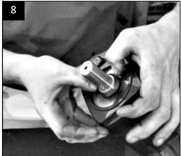
Lubricate thrower with soapy water and fit it on shaft
