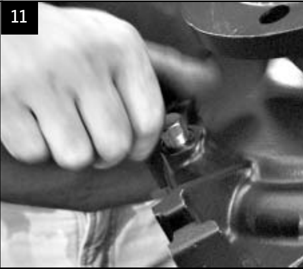
Fit plugs in pump housing
